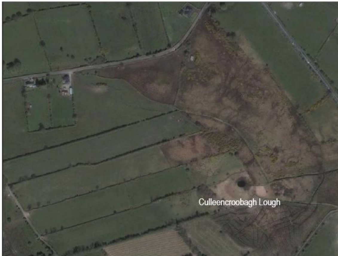
Figure 4.6.1 - Aerial photo of soft ground area around Culleencroobagh Lough, which is a possible swallow hole (Google Maps, 2012)
